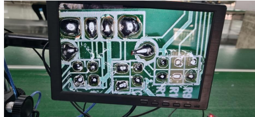
Hand Soldering, SnCu, 280°C covering >95%
