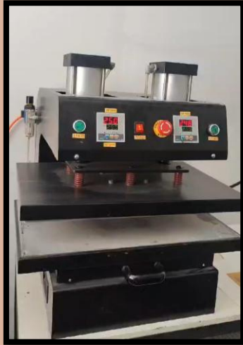
Hot-Press Small to medium production scale
