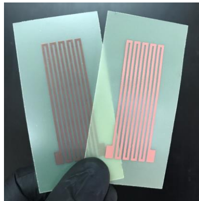
Figure 5 Non sintered (left) and sintered (right) printed pattern
